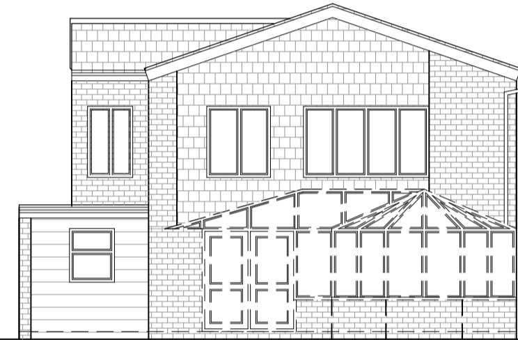
Existing Rear Elevation (Structure Demolished) Refer to Key
